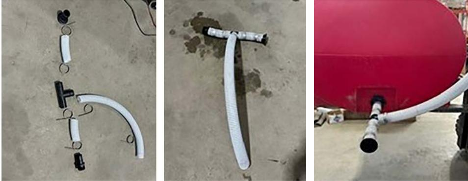
**Step 8:** Ball valve install for intake on pump, then connected to pump intake.
