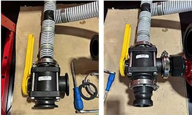
**Step 9:** Ball valve install for intake on pump, then connected to pump discharge.
